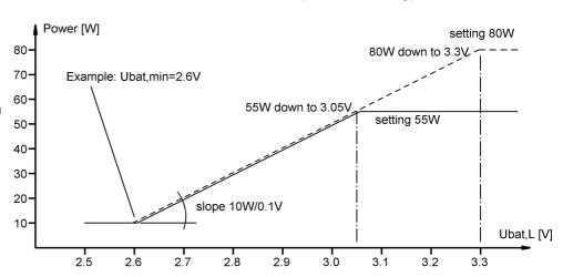
utilization. At UBatMin+ 0.7V a power reduction is activated depending on the actual power setting. The reduction starts when the power selected hits the slope from Ubat,min@10W to Ubat,min+0.7V@80W as shown in the diagram above. With every 0.1V of higher battery voltage (higher charge level) 10W more of power is permitted.
